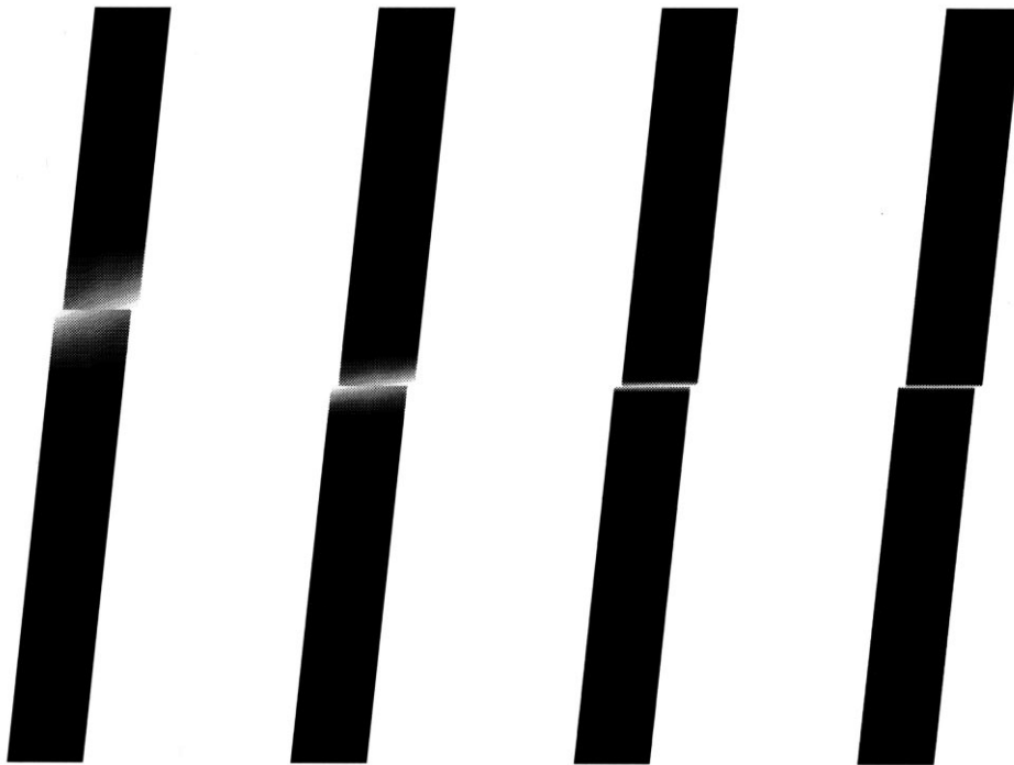
Fig. 12. Deformed configurations and plastic zones for 10, 20, 100, 200 P2 (and 1 I1 ) elements \delta_0=1 .
