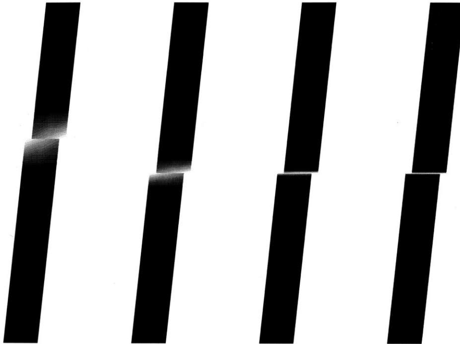
Fig. 10. Deformed configurations and plastic zones for 10, 20, 100, 200 P2 (and 1 I1 ) elements \delta_0=2 .
